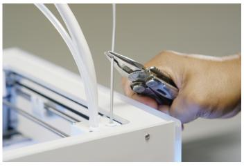
5. Check the color and the shape of the tip of the material that you have pulled out. Compare it with the pictures below to see if it looks correct. If not, repeat this process.
