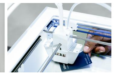
After calibrating the build plate with the first nozzle, the second nozzle needs to be aligned as well, to ensure the heights of both nozzles are set correctly. For this it is only necessary to set the correct height by using the calibration card.
