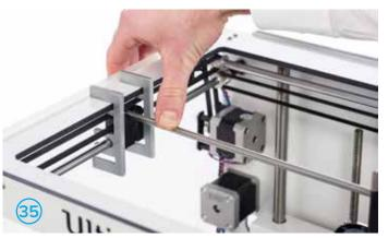
Repeat the steps for the other side of the X-axle and the front and back of the Y-axle. Fig. 36 and 37.
